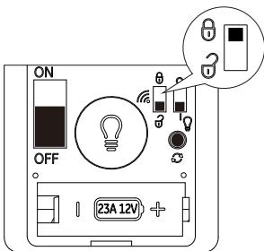
In Case Of Interference With Several Fans, You Can Change The Transmitter Code To Operate A Single Fan Only.
